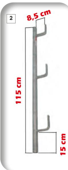
CET ÉLÉMENT PLAQUÉ ASSURE UN COFFRAGE JUSQU'À 40cm ET LA PROTECTION DE L'UTILISATEUR. LA MISE EN PLACE DOIT SE FAIRE TOUTES LES 150cm MAXI ET LE RÉGLAGE DU MONTANT DE DÉPART VARIE ENTRE 0 ET 15cm. CETTE PROTECTION RÉGLABLE SE DÉCOMPOSE PAR:
